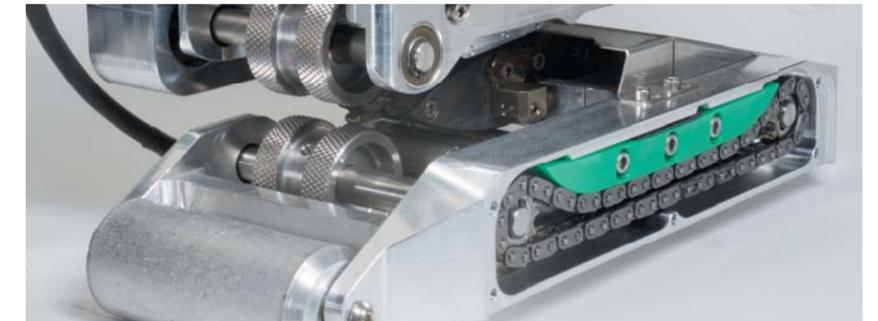
The temperature of the heating wedge is kept at up to 500°C with maximum precision, based on the specs of the used material, after the nominal temperature and the material characteristics for the imminent welding job were entered. The newly developed monitor for current flux to the heater cartridge ensures continuous temperature control. A possible current failure gets detected immediately and a plain-text alert shows on the high-res temperature range-extended character display.
